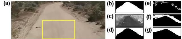
Figure 10. (a) Original image after sky removal and its Otsu's result in (b); (c) negated image and its Otsu's result in (d); (e) Canny edge detection result; (f) Hough transform result; (g) a single mass from the image (f).
